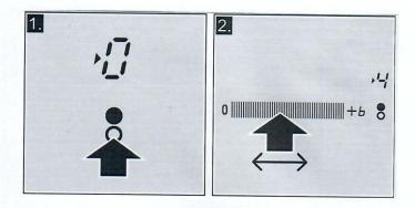
1. Switch on hob with main switch. Touch the symbol for the desired hotplate. The display 0 and an arrow light up.
